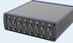
BX8-HD15/ BX8-HD44 Data Acquisition System & Amplifier 8 Channel
