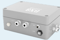
BX8-AS Data Acquisition System & Amplifier 8 Channel
